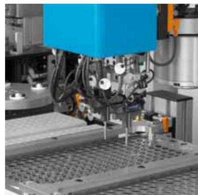
The pictures show an automatic classification machine for selecting on the basis of outer diameter. A twin measuring stand is used to cut the cycle time in half by allowing two parts to be measured simultaneously in a single step. The measuring technology is based on the scanning principle, whereby a pneumatic ring gauge passes over the cylindrical part of the item and measures around 200 points.
