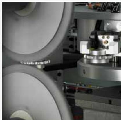
Twin-sided brush units to deburr both faces of a sintered item in a single step
