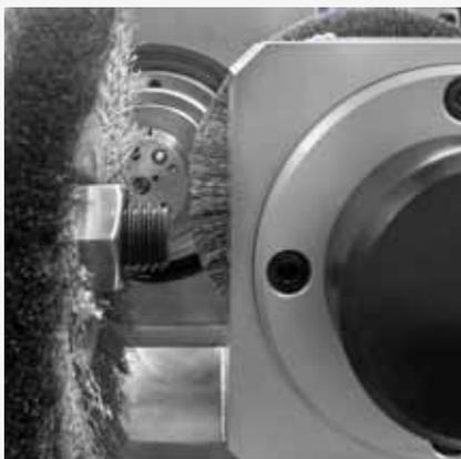
Simultaneous face and outside diameter brush deburring
